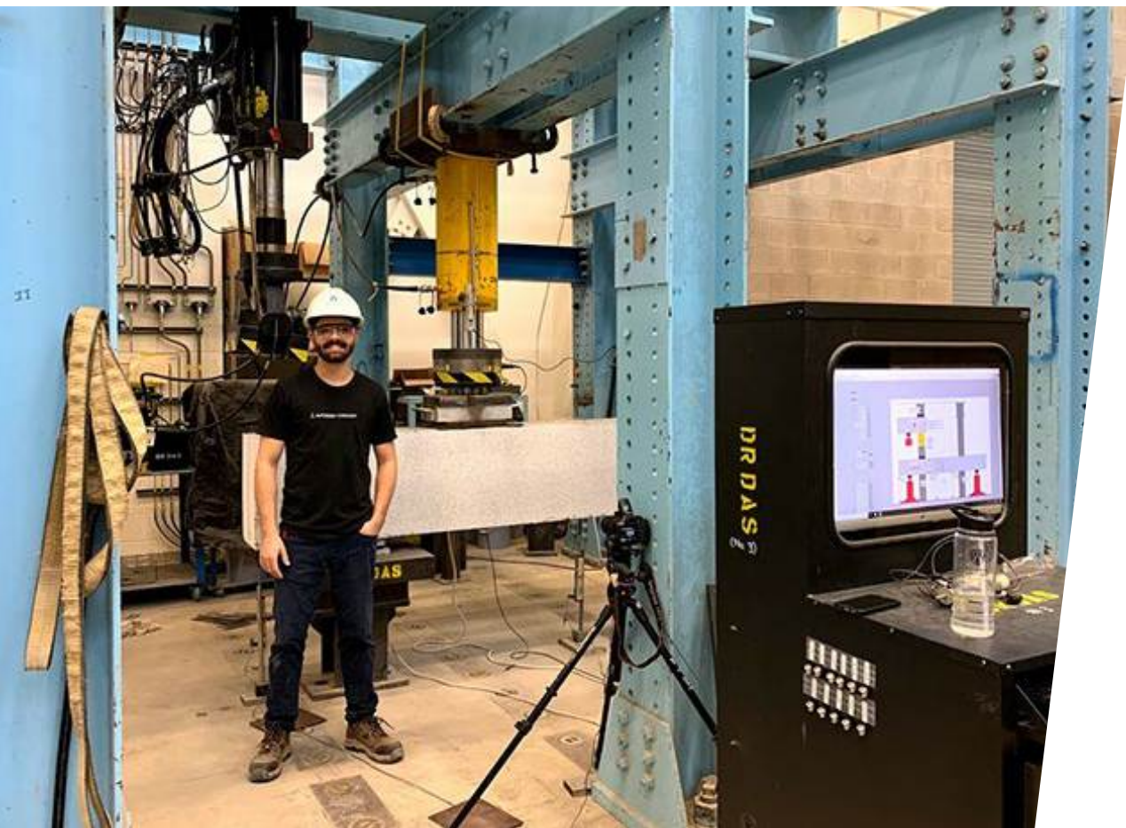
A test set: The black box is the DAQ (data acquisition) system. Courtesy of Dr. Sreekantha Das's Research Group.
