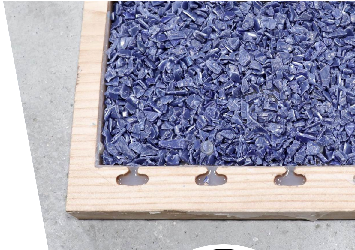
Tile mold, filled with shredded plastic. (above)
