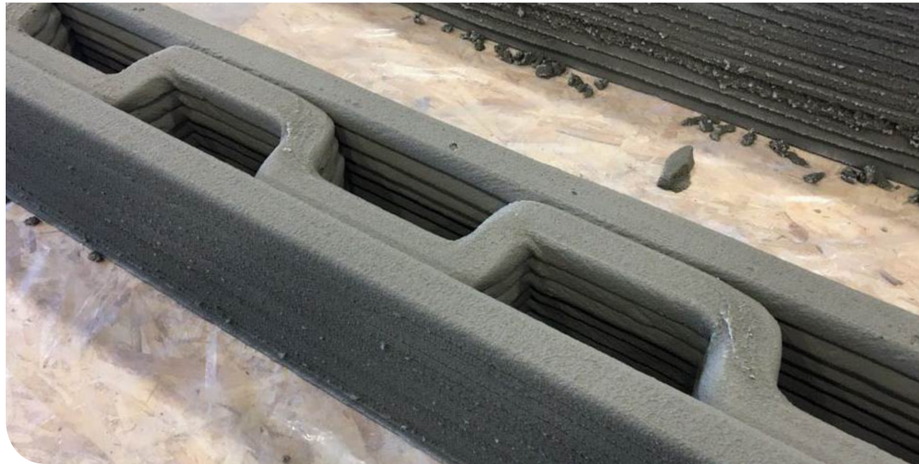
3D-printed wall structure. Courtesy of Apis Cor.
