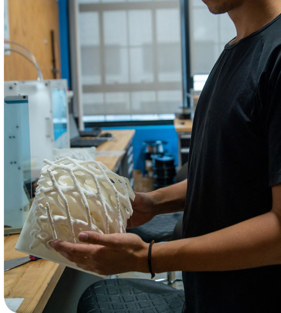
Elliott Santos developed a novel cladding system that could be applied to building facades to provide passive wastewater treatment. Courtesy of Elliott Santos.
